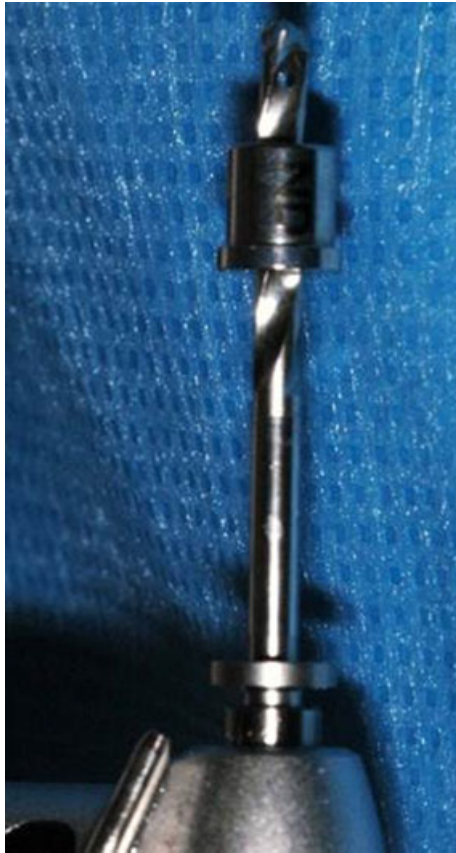
Fig. 8. Drill key on drill. The drill is placed with the drill key in the guide, then the drill moves through the key.
